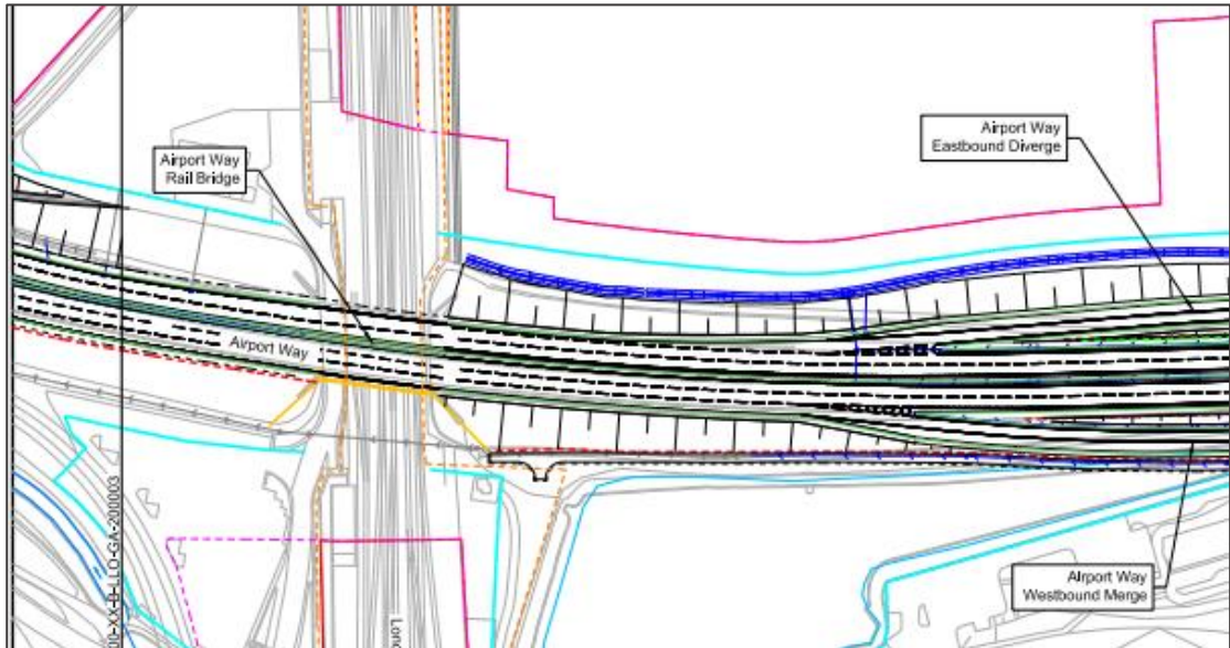
Figure 665: Airport Way Westbound new third lane
